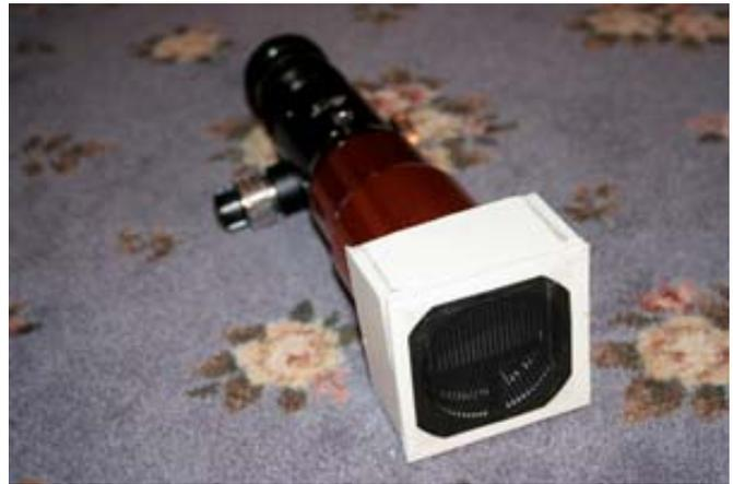
I took the easy way out and printed it to a transparency which is much easier and works just as well. Once you have it mounted onto your scope, point it to a bright star and adjust focus to get the scope near focus through the viewfinder and take a test shot of a few seconds. The test shot will look something like a star with six spikes below.
