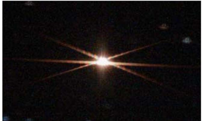
Notice how the center spikes are a bit high or low depending on which side of focus you are on and not centered between the diagonal spikes. Now the goal is to adjust your focus until the side spikes are right in between the diagonal as shown below.
