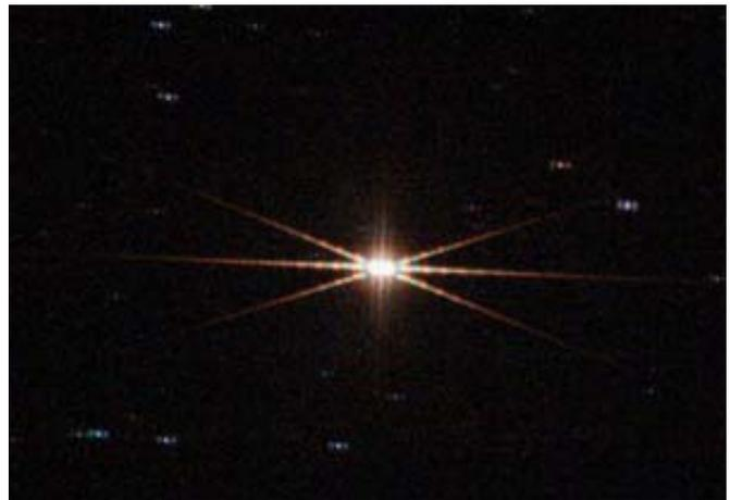
Once this is accomplished remove the mask and your camera is focused and is ready to be slewed to your targets for an evening of imaging.
